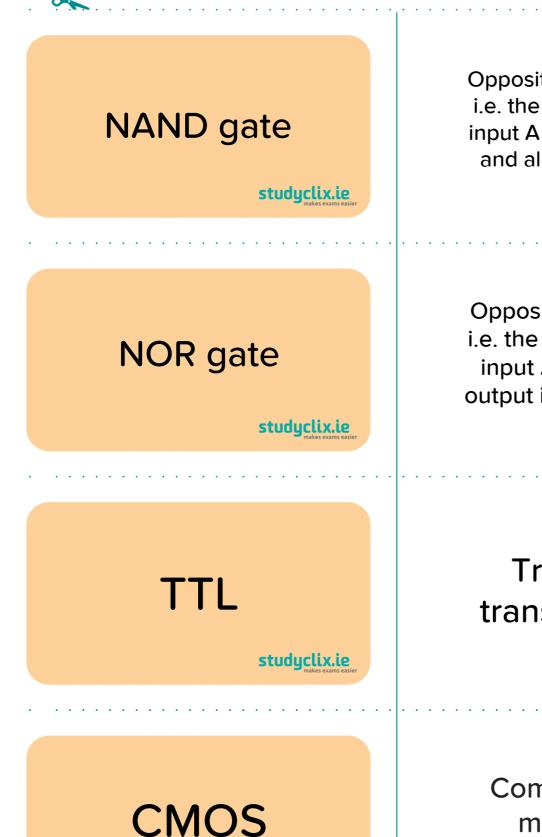
Opposite of an AND gate i.e. the output is 0 when input A and input B are 1, and all other cases the output is 1
